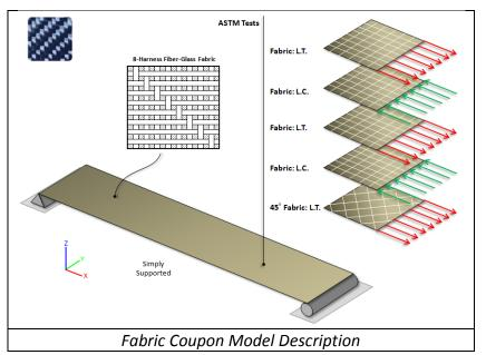
modeled assuming 8HS weaves and representing each weave by three stacked fiber/matrix plies, each containing a different fiber volume ratio, depending on the crimp angle. MCQ-Composites offer a way to calibrate the composite architecture based on the data provided by five ASTM tests.
