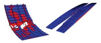
**Impact:** Dynamic analysis coupled with Lsdyna or Abaqus Explicit to replace various impact tests such as crush & crash, bird-strike, drop, compression after impact, etc...
